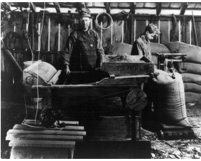
Figure 2. Electricity also brought new technology to the farm. Many farmers built their own machinery, such as this electric-powered feed mixer.
