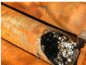
Figure 6. At Lake Ontario in Canada, zebra mussels cling to the inside of a rusty pipe.
